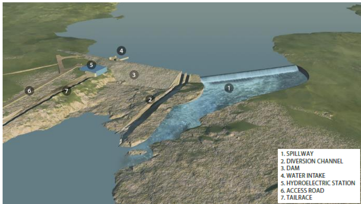
FIGURE 1: ILLUSTRATION OF THE INNAVIK HYDROELECTRIC PROJECT
